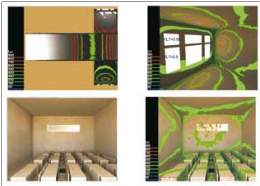
Figure 5 Typical north (top) and south (bottom) side classroom illumination levels in December. Adequate daylight is made available by optimizing window design
